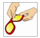
Continue to work the lens into the frame, working from the inner corner across the top, around the side and across the bottom, fitting the keyhole notches securely over the posts. When lens is completely inserted, ensure the gasket grips flat against the lens all around it. Repeat to insert the other lens. Clean lenses (see below) to remove fingerprints and smudges.
