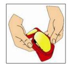
Push the lens forward forcefully to release it from the gasket of the eyepiece.
